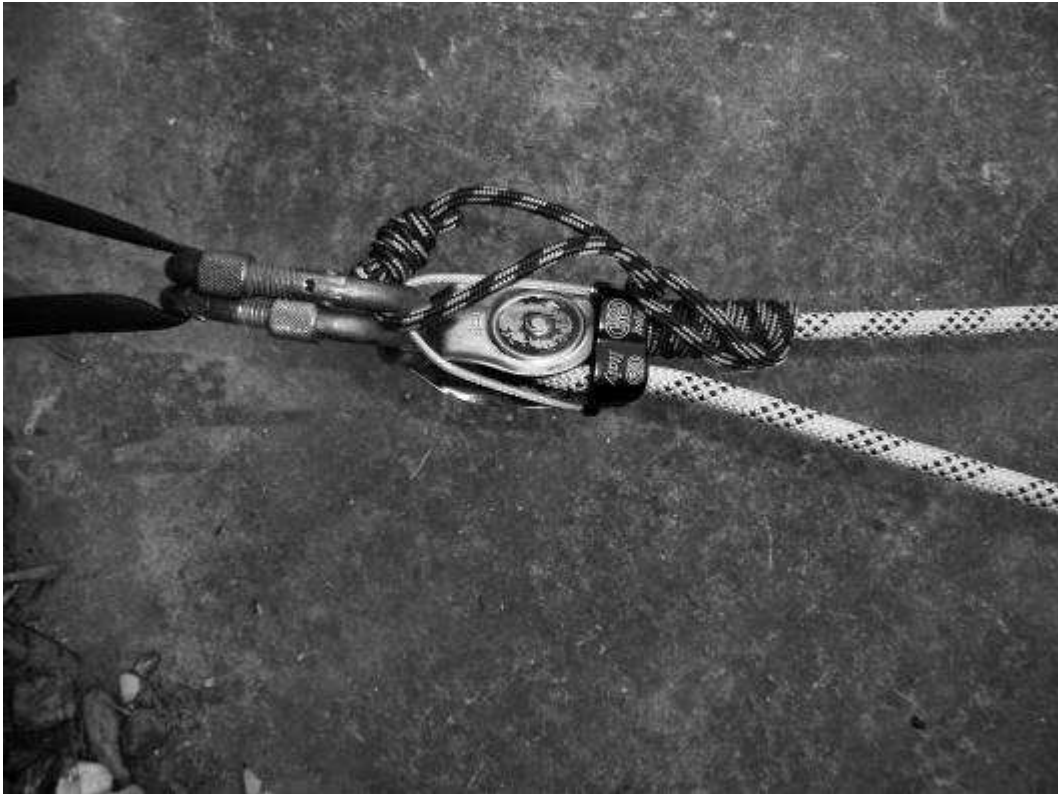
Auto-brake with the rope being hauled
